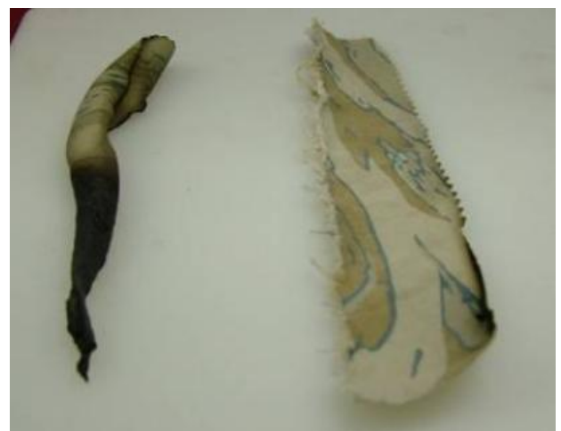
Above are two samples, one was treated with Alexium's Reactive Surface Treatment (RST) and one was not. This sample on the right underwent a single treatment making it self-extinguishing in a fire and super hydrophobic and oleophobic.
