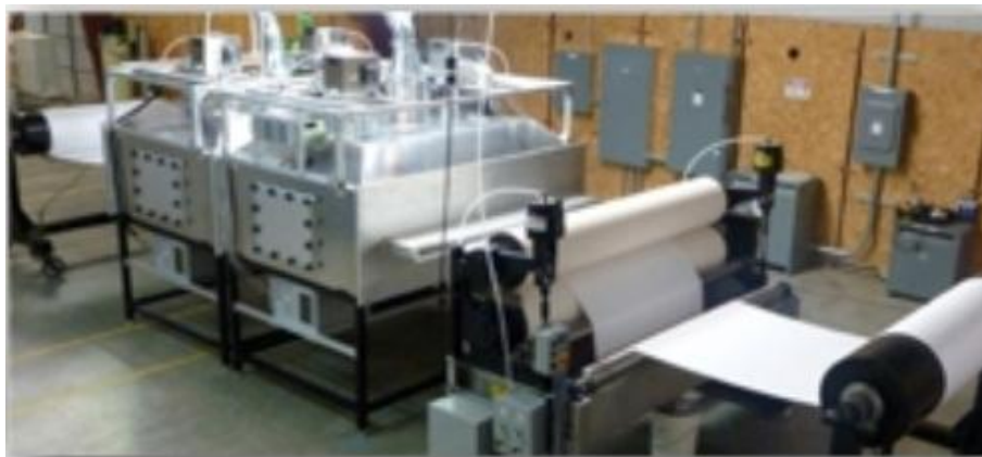
Exhibit 3: Low Temperature Curing Equipment
